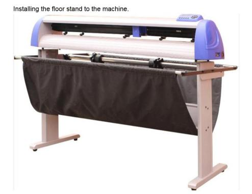
Remove the four nuts from the bottom of the machine mounting bolts and insert the bolts from the bottom of the machine to the top of floor stand by placing the cutter on the stand and aligning the four bolts with the slots in the stand mounting flanges. Secure the machine to the stand using the nuts that were removed from the mounting bolts.
